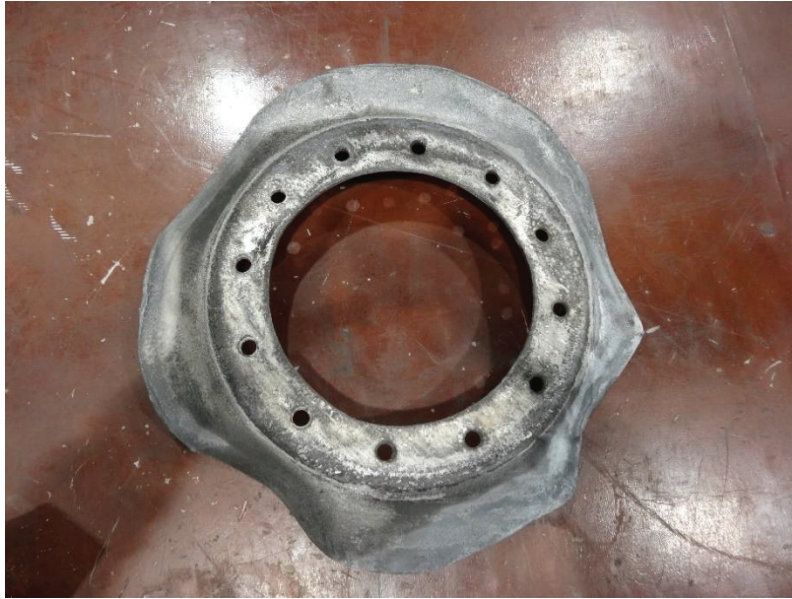
Figure 1. 1 st Gauging Run Gauge Plate
