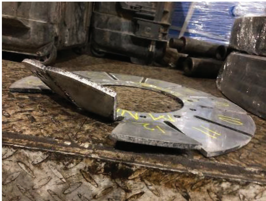
Figure 6. 3rd Gauging run bend plate
