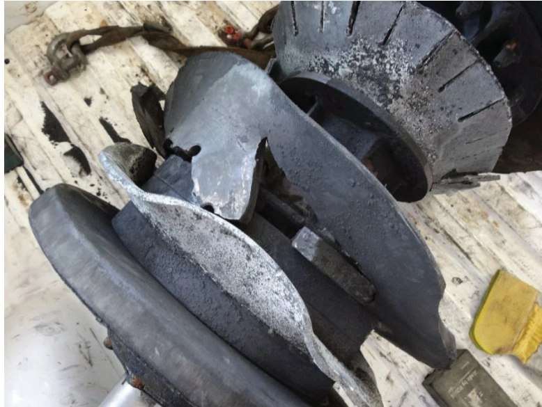
Figure 2. 1 st Gauging Tool Condition
