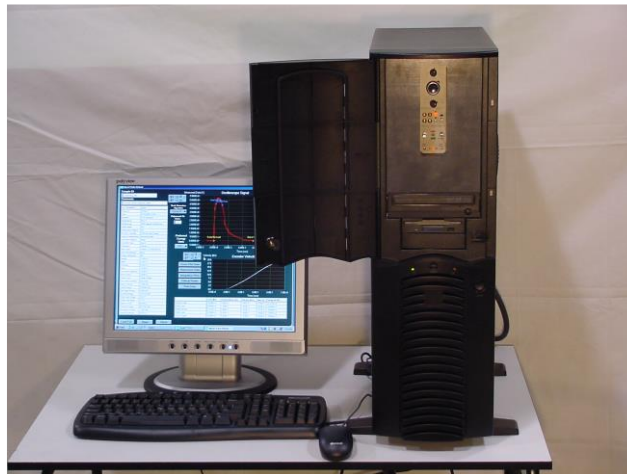
Figure 2 Data acquisition computer with 12 fast acquisition board, encoder board, encoder hardware, and strain gage amplifier. The amplifier provides autobalance, amplifier range selection, and shunt calibration for periodic calibration checking. The amplifier is capable of a wide range of amplification settings for the research environment needs.
