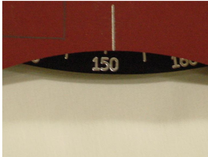
Figure 3 Close up of the latch angle being set for 151 degrees.
