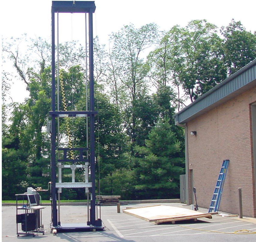
Figure 15 High energy capacity (10,000 ft-lbs) drop tower for impact testing of concrete highway abutments.
