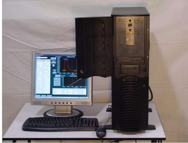
Figure 2 Data acquisition computer with 12 bit fast acquisition board, encoder board, encoder hardware, and strain gage amplifier. The amplifier provides autobalance, amplifier range selection, and shunt calibration for periodic calibration checking. The amplifier is capable of a wide range of amplification settings for the research environment needs.
