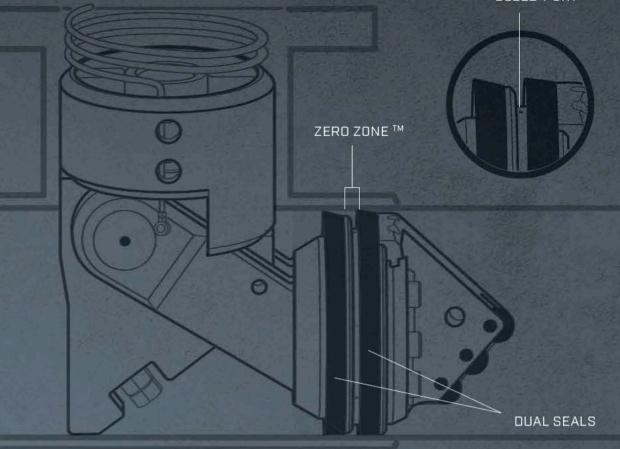
SIZES (inches) Single tap reduces costs Dually / The second sec and saves time. 8" 24" • Simple design/single pivot for 10" 26" cleaner entry and easier removal 12" 30" 16" Easy-to-replace sealing 36" Double Block & Bleed Line Stop System elements mean jobsite flexibility. 20" 42" NACE-compliant materials. TEMPORARY JOB COMPLETE THE PLUGGING LINE STOP AND PIPELINE IS HEAD IS COMPLETION PLUG IN PLACE PIGGABLE LOWERED WITH COUPON SET
