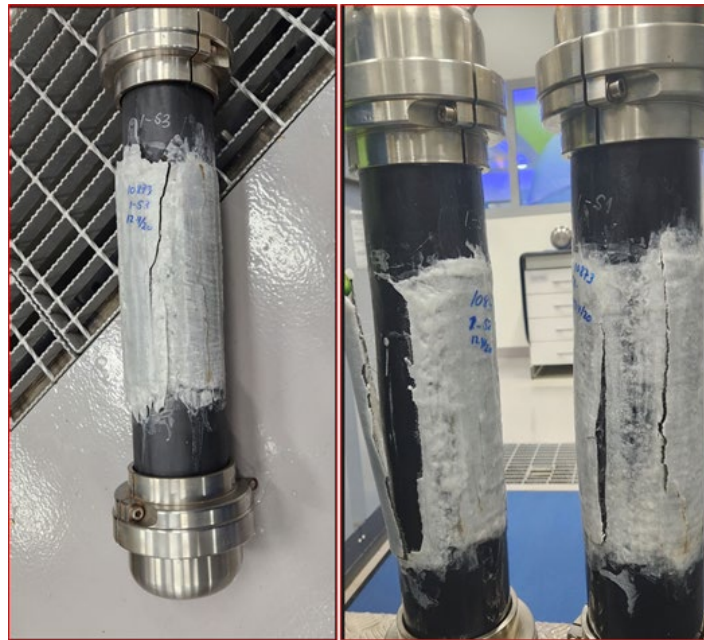
Figure 4. Primary Test – Failure Pipes for HPT test at 20 °C
