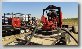
GCPS is equipped to provide and operate 'fit for duty' pumps, specifically sized for your desired flow rate to fill your pipeline in preparation for hydrostatic testing, cleaning pigs, ILI tools, or displacing the existing product from the line with water during the filling process.
