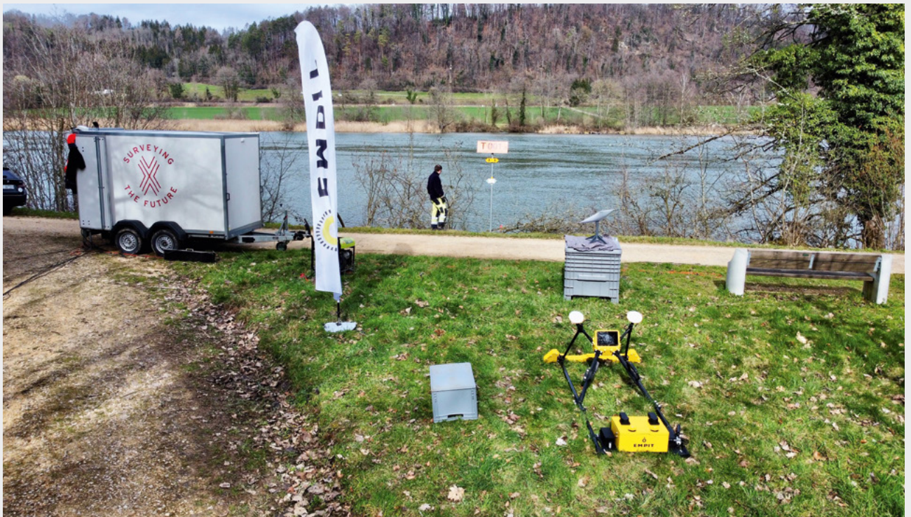
Figure 4: Measurement setup for the CMI. The trailer on the left contains the signal generator. The sensor arrays are integrated into the portable detector (yellow), and above the detector is the Starlink antenna, which sends the large amount of data directly to the cloud for immediate processing.
