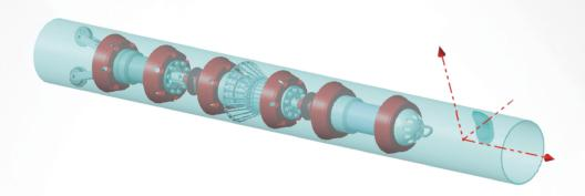
An Inertia Mapping Unit (IMU) provides the actual spatial of tool movement used for this purpose. The IMU consists of accelerometer and gyroscope which provides data which can be then grafted to the X, Y and Z coordinates on a time scale basis.
