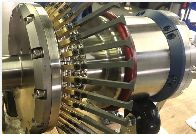
Onboard pipeline geometry assessment (caliper) and onboard Inertial Measurement Unit (IMU) for pipeline XYZ mapping.
