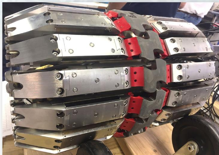
Magnetizer body features 'S-shaped' proprietary sensor design.
