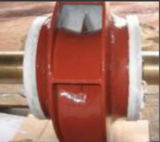
Bronze pump rotor refurbishment
