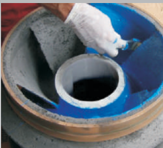
Coating of pump rotor
