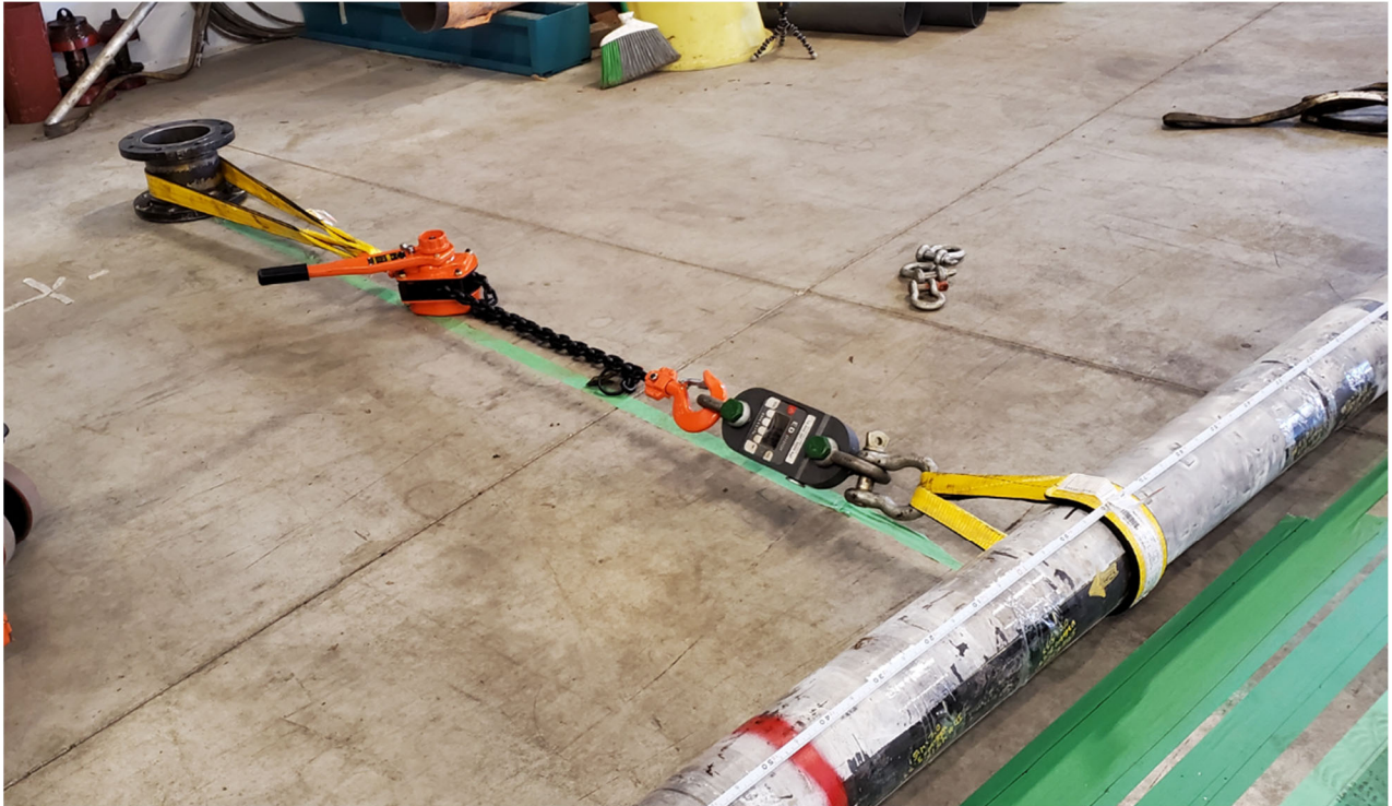
Figure 3 - Pipe simply supported and point loaded at each CSCC cluster location introducing bending stress
