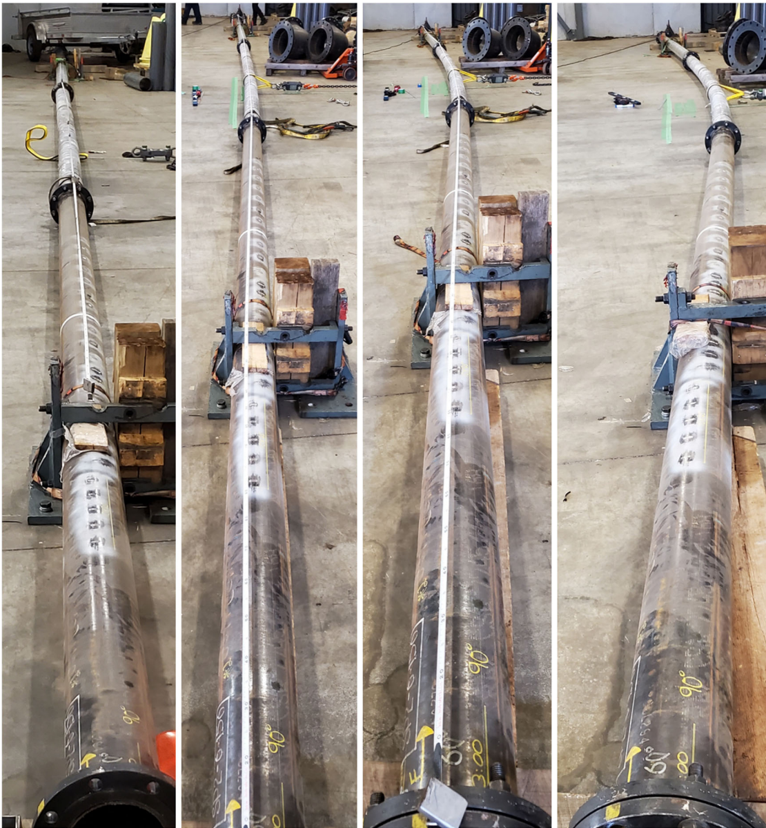
Figure 7 - Bending stress introduced by displacing the test pipe up to 16" from its straight rest position
