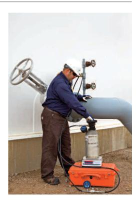
The *Tracer Tight* service works by inoculating a tank or pipeline with a small amount of tracer gas. Probes are installed under a tank floor or along buried piping that can collect soil vapor samples for analysis by a Linde expert technician. If a leak is present, it is easily detected by gas chromatography.
