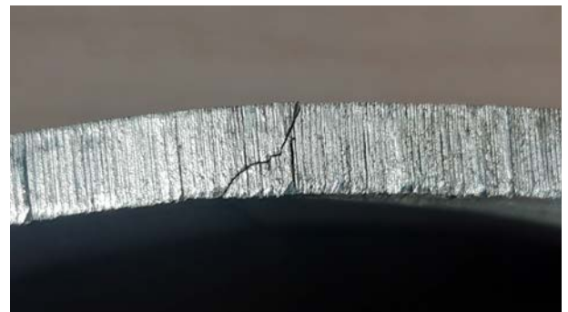
Cross section of an internal hook crack in an ERW long seam after a freeze break.
