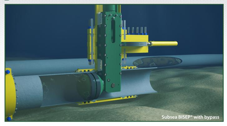
The BISEP when deployed subsea provides the highest level of hot tap installed pipeline isolation in the industry. Complying with all relevant subsea isolation guidelines, the BISEP ensures safe worksite conditions for divers from breaking containment to reinstatement.
