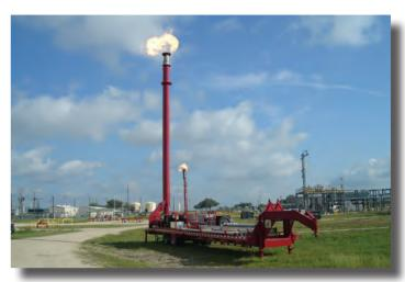
rigged up and ready to go in a matter of minutes. This eliminates costs associated with air compressors, cranes, or other equipment that might be required with other flare stacks on the market.
