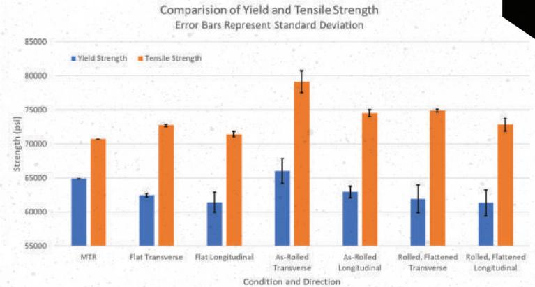
Figure 1: Comparison of Yield and Tensile Strength
