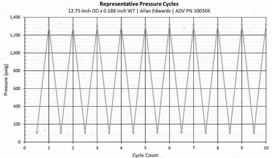
Figure 3-6: Ten (10) Pressure Cycles for the 12" AE Type B Reinforced Samples
