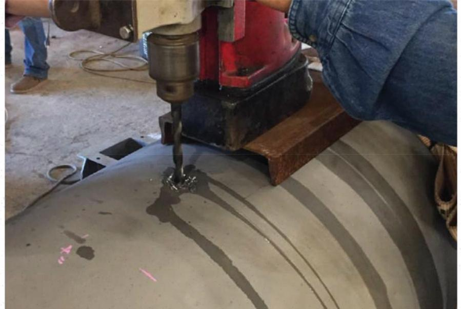
Figure 1: Installation of 1/2-inch holes into carrier pipe
