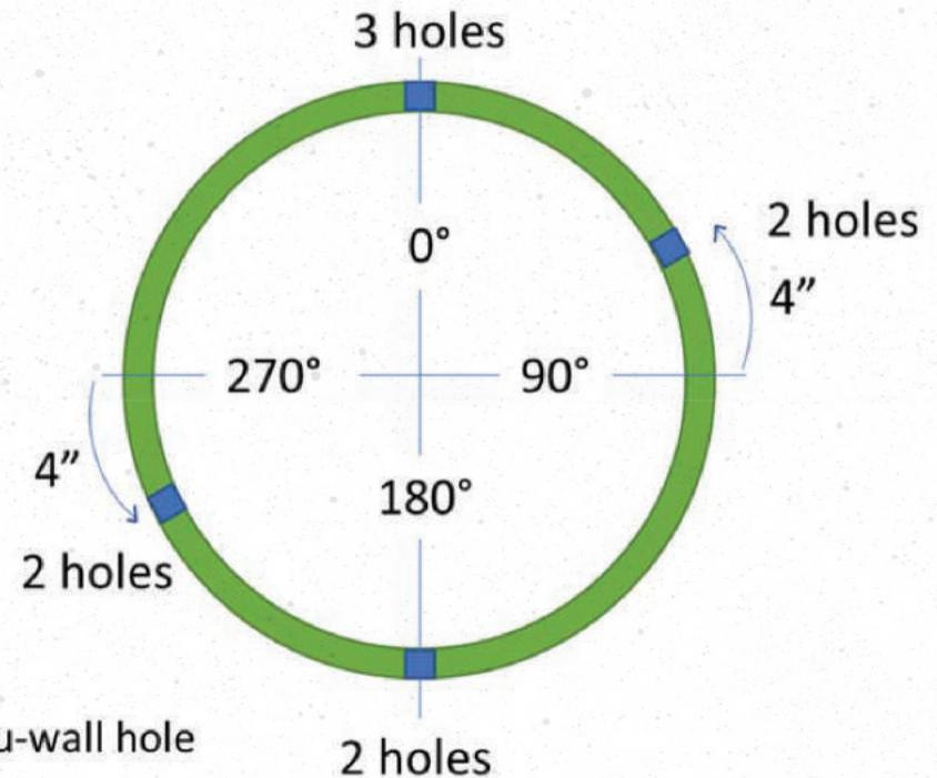
Figure 2: Locations of the nine (9) 1/2-inch thru-holes in carrier pipe
