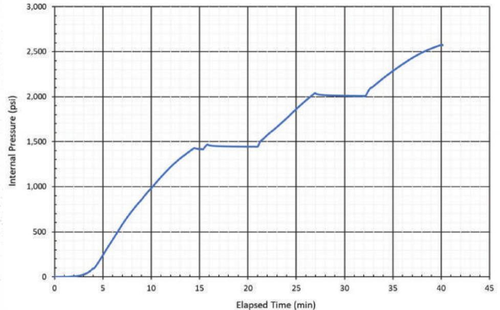
Figure 5: Internal pressure vs. elapsed time for 24-inch Type-B repair sleeve burst test
