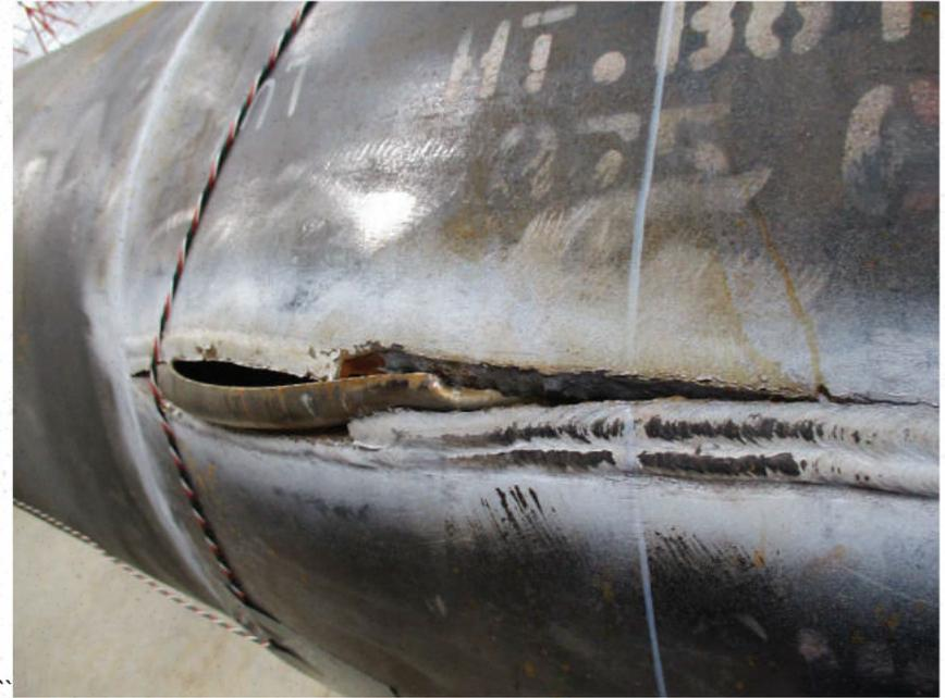
Figure 8: Close-up of burst test failure location – failure pressure of 2,578 psig (126% SMYS)
