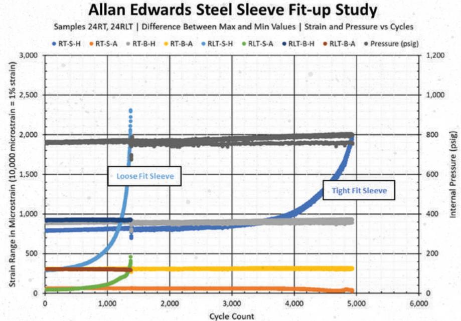
Figure 5: Strain and internal pressure vs. cycles for both Samples 24RT (tight) and 24RLT (loose)
