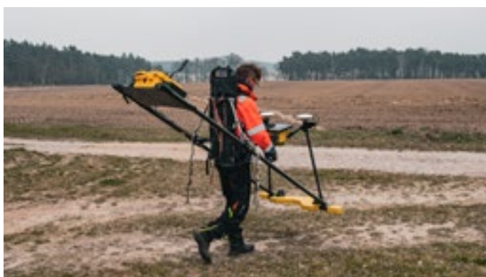
Figure 3: The Current Mapper system during inspection
