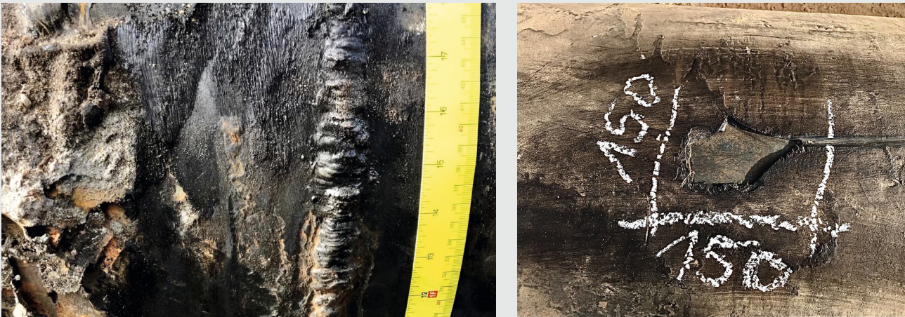
Figure 6: Girth weld anomaly detected with CMI (left) and coating holiday (right)
