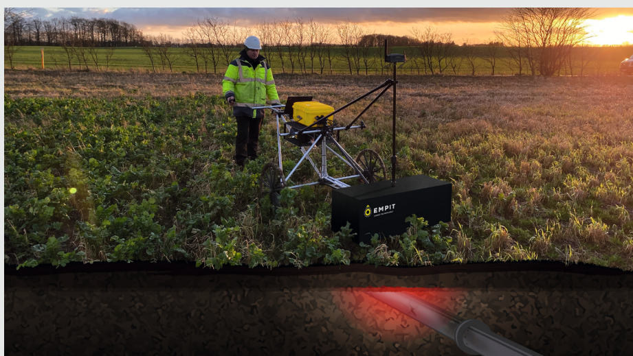
Figure 3: The Field Rover of the CMI Inspection System
