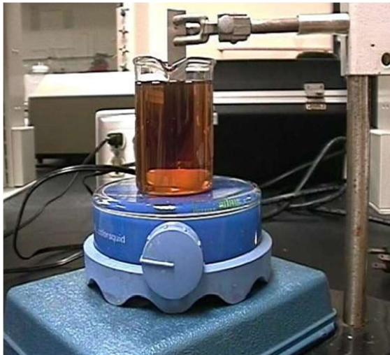
FIGURE 2. LABORATORY BENCHTOP SET-UP FOR COUPON IMMERSION TEST.
