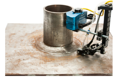
Phased Array Nozzle Inspection
