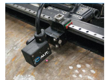
Laser Mapper Surface Scanning
