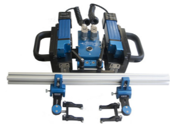
2-Axis - Weld exams / Line B-Scans
