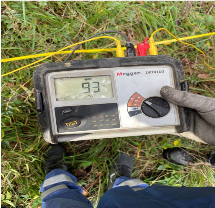
FIGURE 12. Resistance measured by the Megger Soil Resistivity Tester
