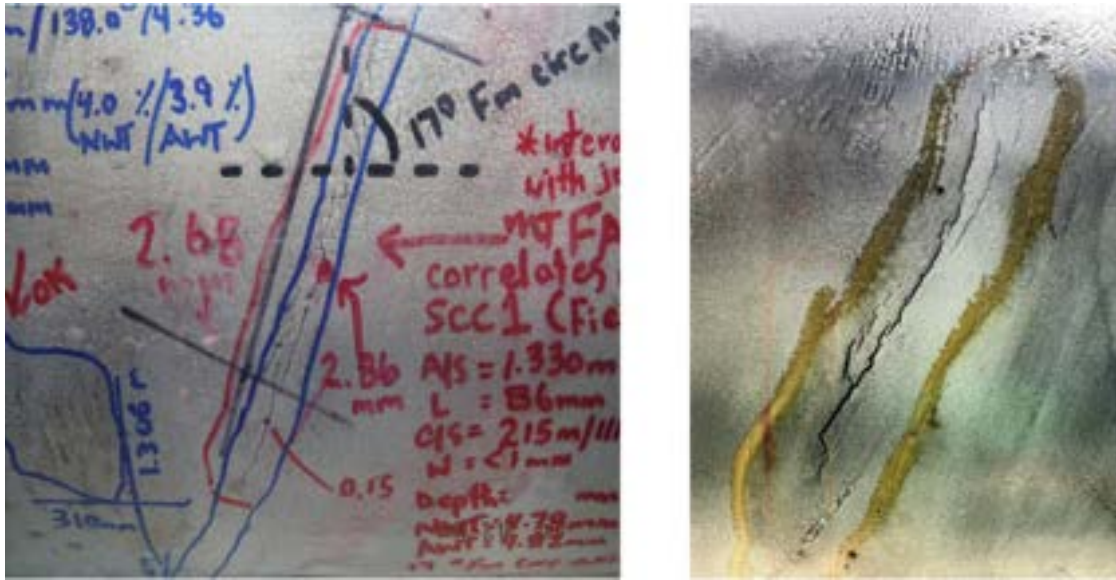
Figure 2. Example of CSCC Features Located at 17° and 27° off the Pipe Circumference.
