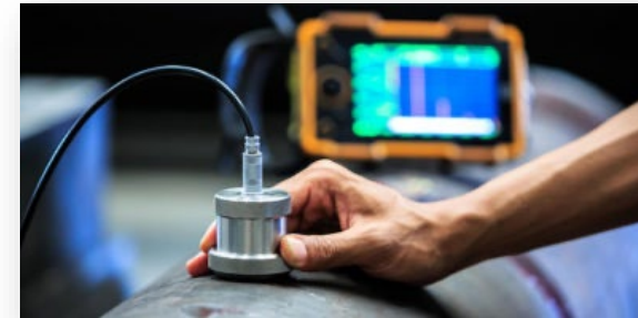
Ultrasonic Testing (UT)
