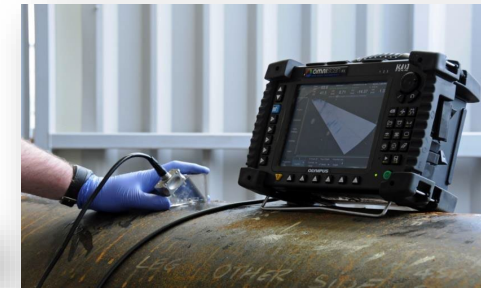
Phased Array UT
