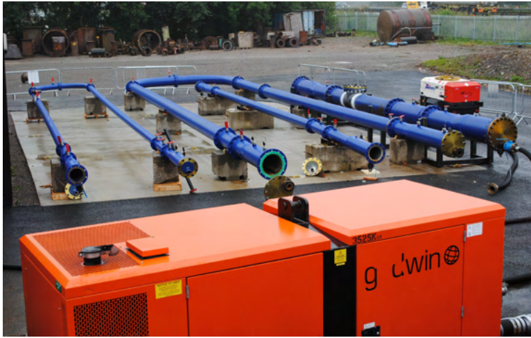
Test loop for proof testing of pigs at iNPIPE PRODUCTS facility
