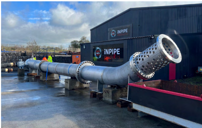
36" Pigging System - FAT Testing & Commissioning at iNPIPE PRODUCTS facility
